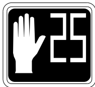
PERSON WALKING INTERVAL FLASHING UPRaised HAND INTERVAL STEADY UPRaised HAND INTERVAL PEDESTRIAN SIGNAL MODULE WITH COUNTDOWN DETAIL B
