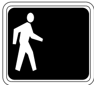
PERSON WALKING INTERVAL STEADY UPRaised HAND INTERVAL PEDESTRIAN SIGNAL MODULE WITHOUT COUNTDOWN DETAIL C
