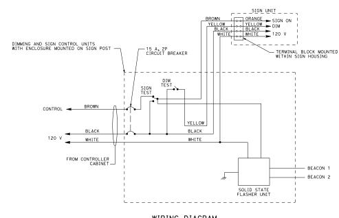
WIRING DIAGRAM EXTINGUISHABLE MESSAGE SIGN
